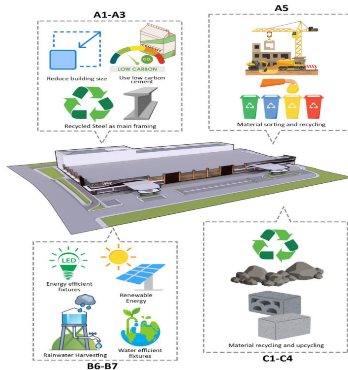
Figure 5. Design strategies for minimizing environmental impacts across building life-cycle stages; economic feasibility and cost–benefit performance requires further evaluation through life-cycle cost analysis.
