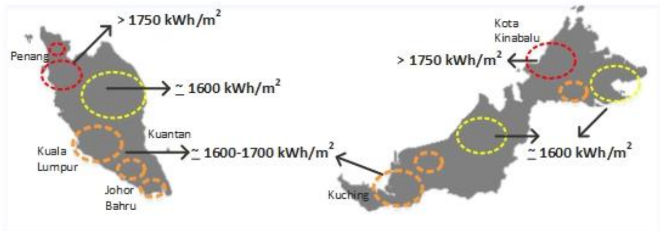
Figure 5. Solar intensity distribution in Malaysia, redrawn based on solar intensity contour map retrieved from Ahmad et al. (2013).
