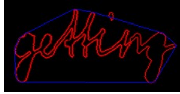
Fig. 9: Computation of convex hull on a from outer contour of Roman script component
