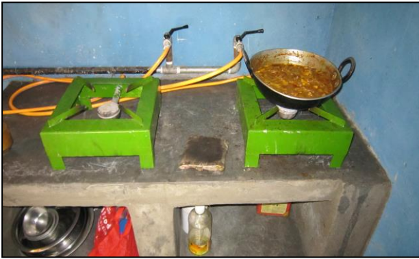
Figure 9 The stove burns and food is cooked using the gas produced by the system.
