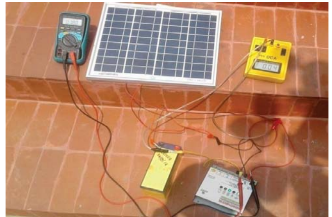
Fig.10 Solar panel, DC Ammeter, Voltmeter, Battery, & Charge Controller used for data collection.
